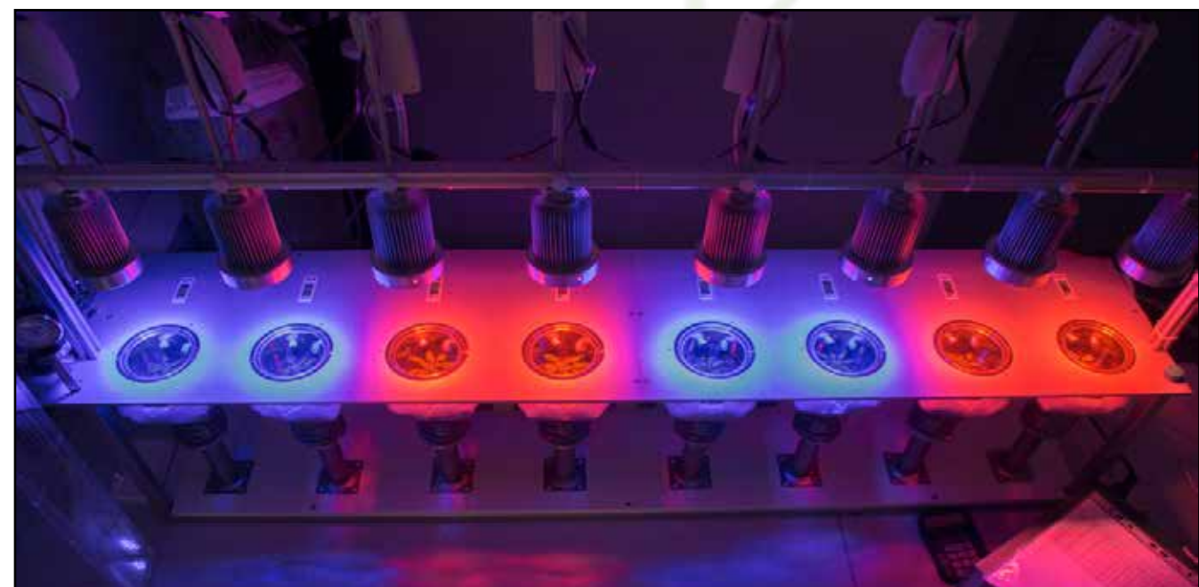
Figure 26. Gas exchange analysis for phenotyping Arabidopsis in a multi-cuvette system since 2006 (University of Tartu, prof Hannes Kollist). Photo by Kaspar Koolmeister.
